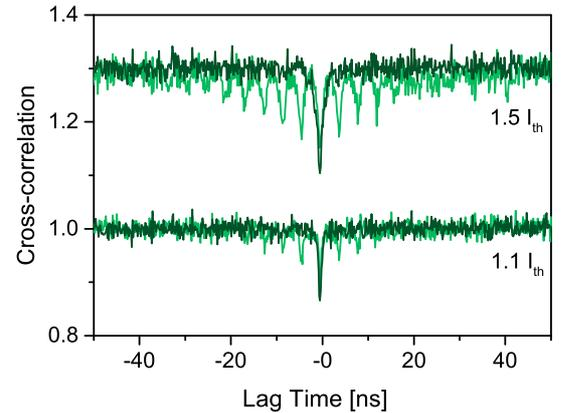
Figure 2: Crosscorrelation of strong and weak modes for two different bias currents. The curves corresponding to  $1.5 I_{th}$  have been shifted upwards for clarity. The scenarios without and with feedback are plotted in the respective colors of the input-output curves (see Fig. 1).
